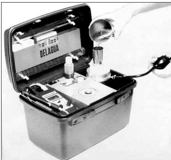
Plate 7.30 DelAgua portable water testing kit. Courtesy of Robens Centre for Public and Environmental Health.
