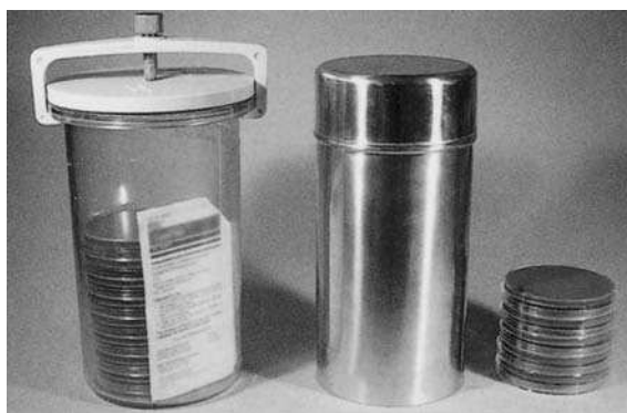
Plate 7.5 Systems for culturing in carbon dioxide. The jar can be used with chemicals which provide a carbon dioxide (CO 2 ) enriched atmosphere and the tin with a candle to provide CO 2 conditions (see text). Reproduced from Laboratory diagnosis of sexually transmitted diseases , WHO 1999, with the permission of the World Health Organization.
