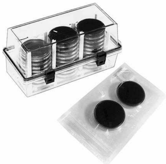
Plate 7.4 Left: BD GasPak container system. Right: BD GasPak pouch system. Courtesy BD Diagnostics.
