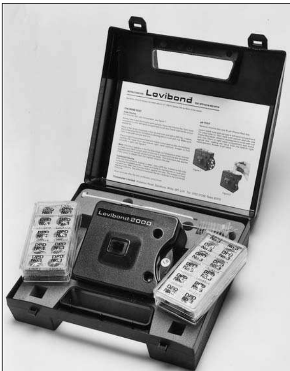
Plate 7.32 Lovibond comparator and DPD tablets for chlorine testing. Courtesy of The Tintometer Ltd.
